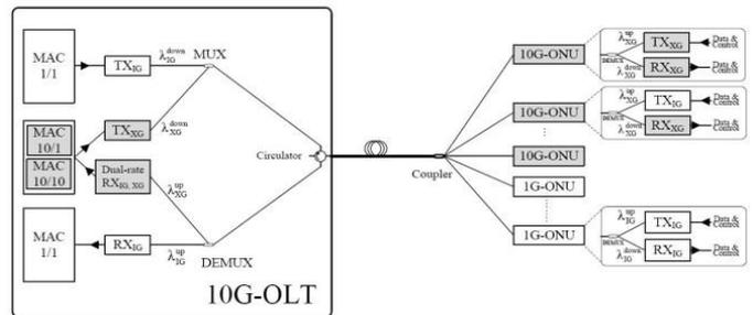
Fig. 4 A typical network architecture for the co-existence of 1G
