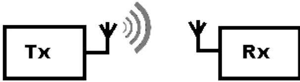
Fig. 9 SISO - Single Input Single Output
