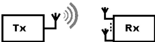
Fig. 10 SIMO - Single Input Multiple Output
