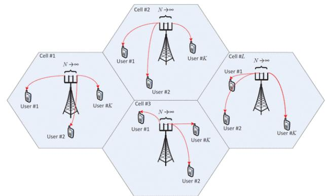
Fig. 12 Downlink of a multi-cell massive MIMO system.
