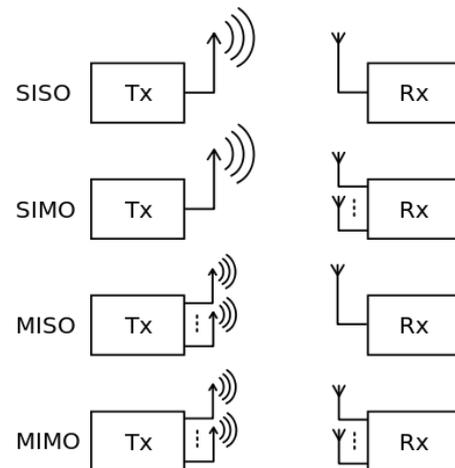
Fig. 1 Understanding of SISO, SIMO, MISO and MIMO
