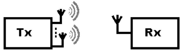
Fig. 11 MISO - Multiple Input Single Outputs
