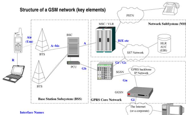
Fig. 5 Structure of GSM Network
