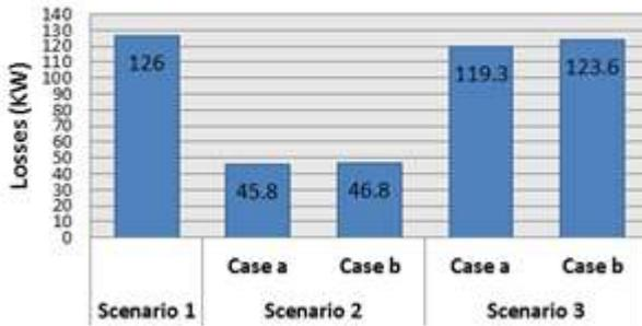
Figure 5: Power losses of line12 with DG unit
