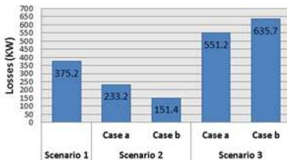
Figure 7: Total feeder power losses with different DG units
