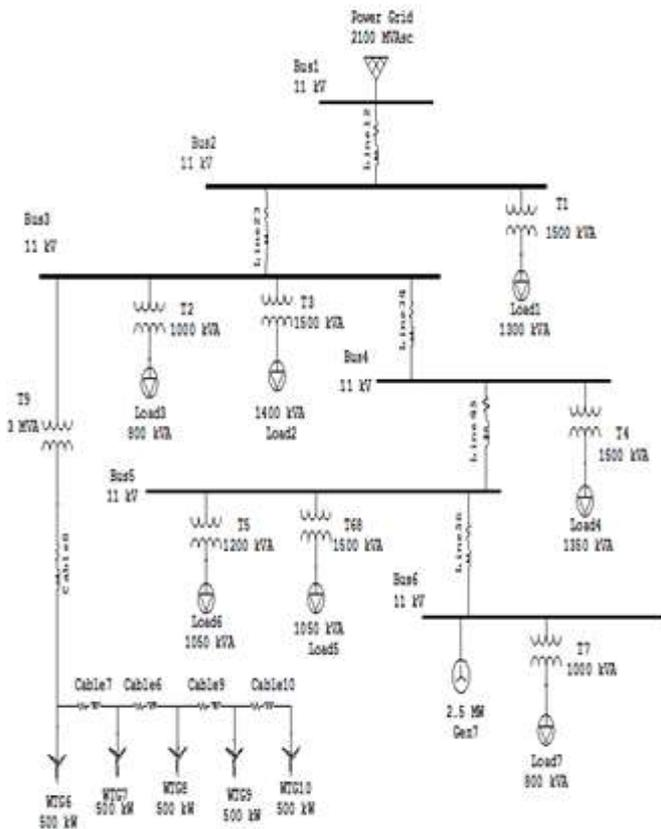
Figure 1: Single line diagram of the test feeder
