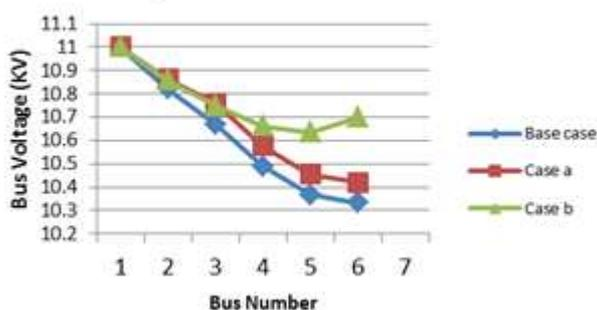
Figure 4: Voltage profile of all buses in Scenario 3
