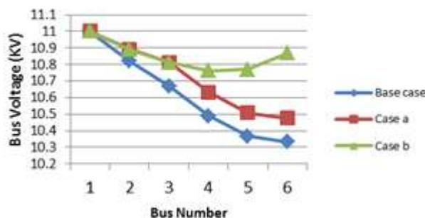
Figure 3: Voltage profile of all buses in Scenario 2
