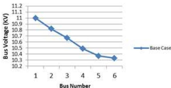
Figure 2: Voltage profile of all buses in Scenario 1
