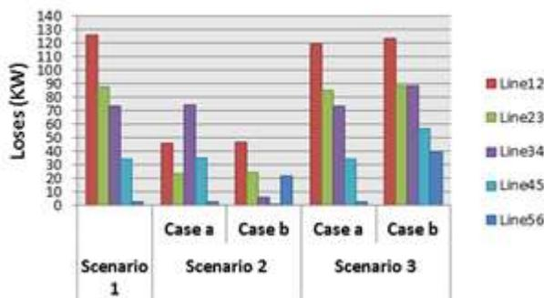
Figure 6: Power losses of all lines with different DG units
