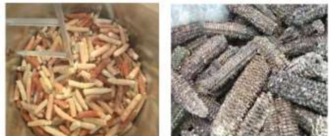
Figure 2. Filter Media (Maize Cobs)
