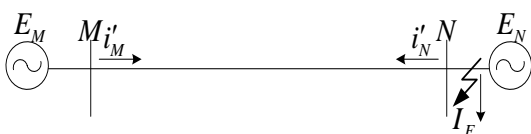
Fig. 2 External fault on distributed transmission line model
