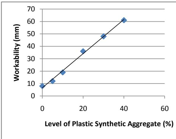
Figure 4. Workability of Concrete vs Level of PSA (%)
