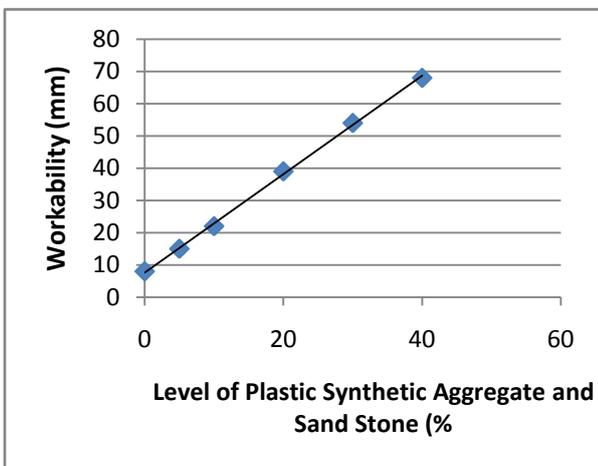
Figure 6. Workability of Concrete vs Level of PSA/SS (%)
