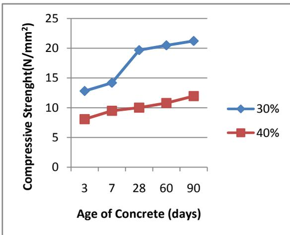
Figure 5. Compressive Strength of PSA/SS concrete vs Ages of concrete 30%-40%
