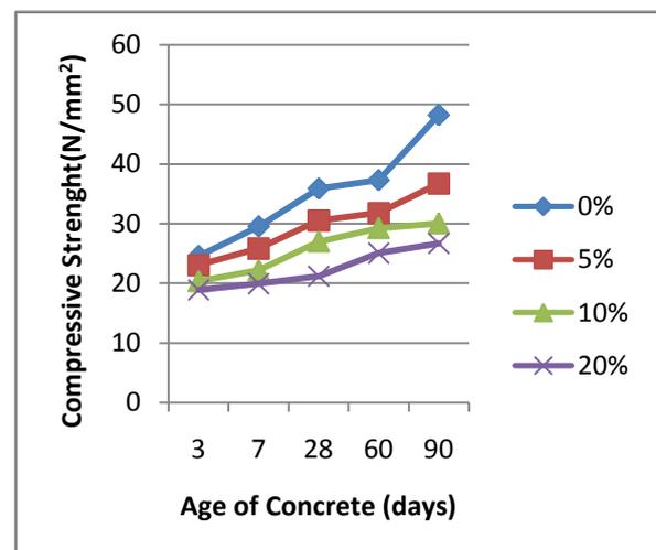
Figure 3. Compressive Strength of PSA/SS concrete vs Age of Concrete 0%-20%
