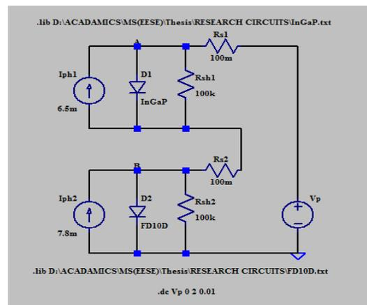
Fig. 4. LTspice model of double junction solar cell
