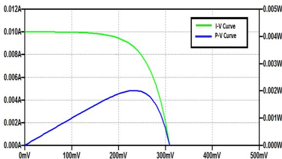
Fig. 3. I-V and P-V Curves of Solar Cell
