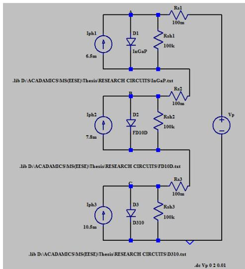
Fig. 6.LTspice model of triple junction solar cell
