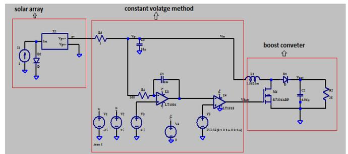
Fig. 9.LTspice model of CV method
