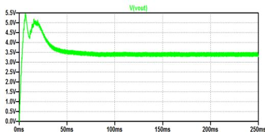
Fig. 12. Output voltage from boost converter
