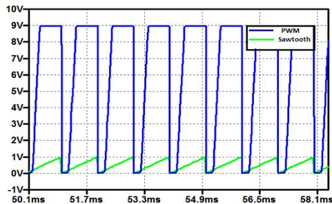
Fig. 10. Generating PWM for switch with constant voltage method
