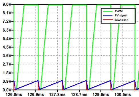
Fig. 16.Generating PWM for switch with P&O method
