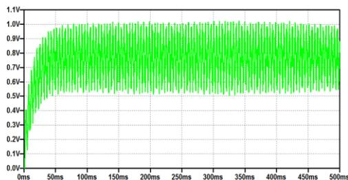
Fig. 11. Output voltage from solar cell
