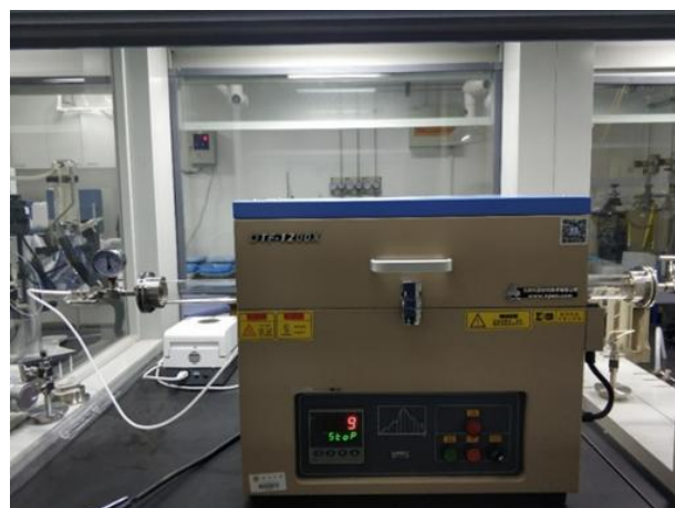
Figure 1. tubular furnace reactor used in experiment
